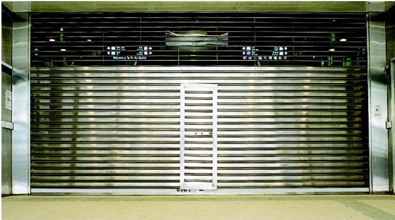
E Electrical isolating device can be added to wicket door to prevent unlossened wicket door from rolling up and damaging the shutter curtain.
