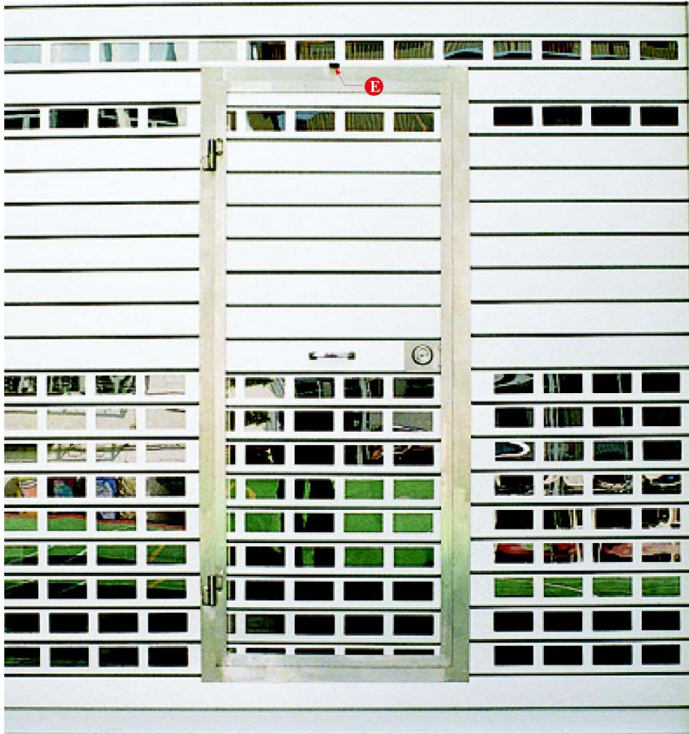
E Electrical isolating device can be added to wicket door to prevent unlossened wicket door from rolling up and damaging the shutter curtain.
